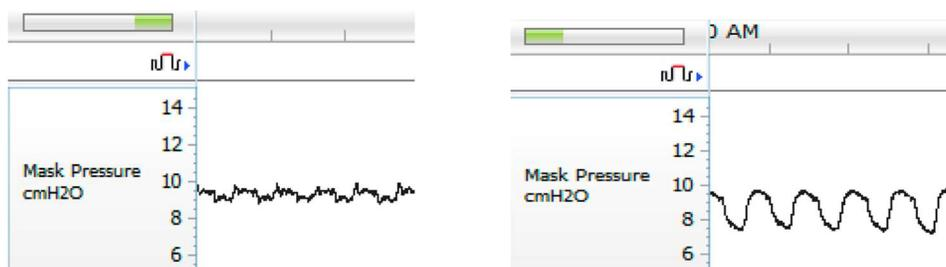
**Figure 5:** Mask Pressure During Respiratory Cycle without V-Com (left) and with V-Com (right)
