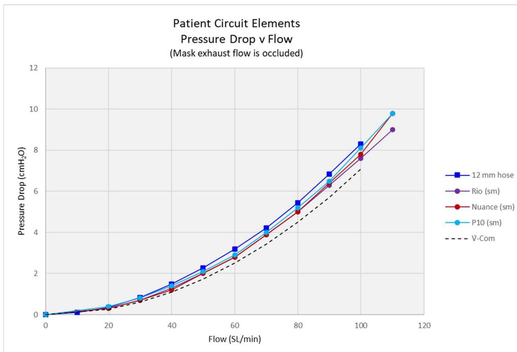
**Figure 3:** Pressure-flow curve of V-Com™, 12 mm circuit hose, and 3 nasal pillow masks with small cushions. At high flow (during inspiration) a large pressure drop occurs (reducing IPAP). At low flow (during expiration) minimal pressure drop occurs (preserving EPA)
