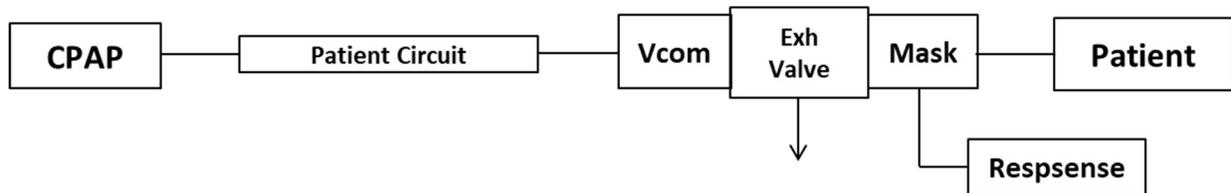
**Figure 7:** Schematic for CO<sub>2</sub> experiments. Note that Respsense is a capnography monitor from Nonin.
