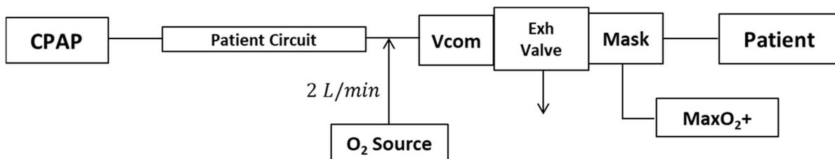
**Figure 8:** Schematic for FIO<sub>2</sub> experiments. Note that the MaxO<sub>2</sub>+ is an oxygen analyzer from Maxtec.
